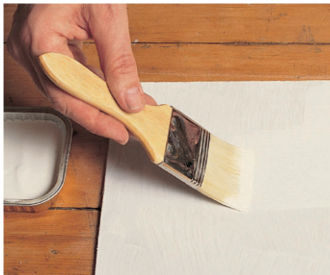
3. Repeat steps 1–2 using brushstrokes painted at right angles to the previous ones. Always sand between coats.
